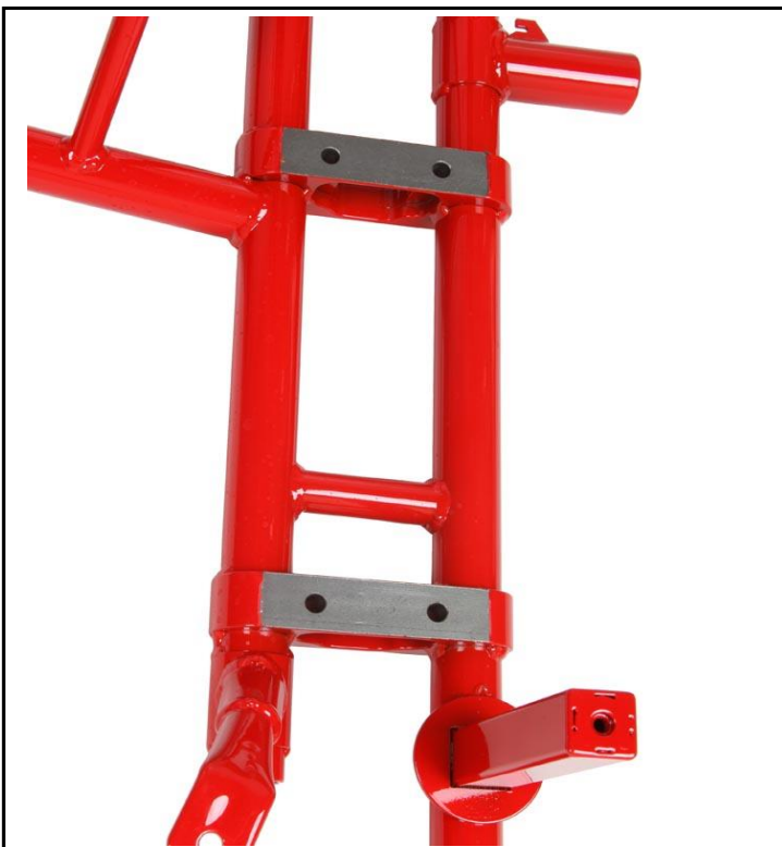
Photo from above of the frame with the section of the engine mount
